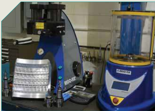
Northeast Tire Mold's REGO-FIX powRgrip unit, tool balancing system and about 200 powRgrip toolholders are critical to shop's direct machining of tire molds.
