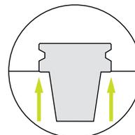
Higher toolholder stiffness due to taper (AT1) and face contact with REGO-PLUS holders.\*
