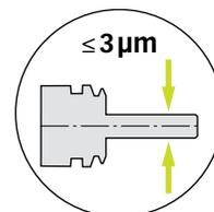
Total system runout TIR  $\leq 3\ \mu\text{m}$  at  $3\times D$ .
